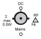
The receiving signal is fed into the RF input socket (BNC socket). It delivers also the remote power feeding voltage.
